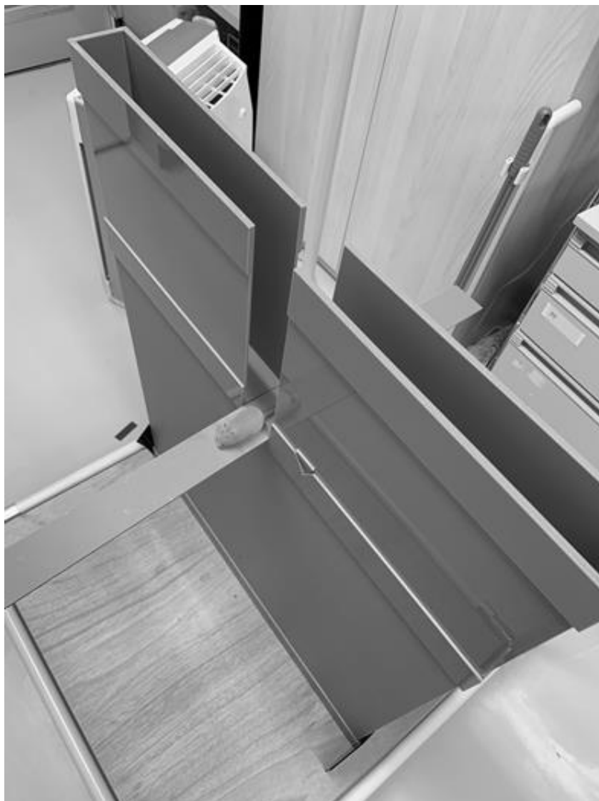
Fig.1. Elevated Plus Maze Test. The elevated plus maze consisted of a plastic criss-crossed open arm ( 50 \times 10 cm), a closed arm ( 50 \times 10 \times 40 cm), and a central square ( 10 \times 10 cm) with a 60 cm high device.
