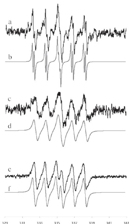
Figure 2 ESR signals of  $\text{HO}^\bullet$  and  $\text{O}_2^{\bullet-}$  adduct of EDPHPN and their computer simulation. (a) shows EDPHPN/ $\text{HO}^\bullet$ , (b) shows computer simulation of (a), (c) shows EDPHPN/ $\text{O}_2^{\bullet-}$ , (d) shows computer simulation of (c), (e) shows EDPHPN/ $\text{O}_2^{\bullet-}$  in pyridine, and (f) shows computer simulation of (e).
