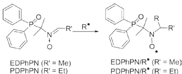
Scheme 3 Spin Trapping of Several Radicals with Linear Spin Traps
