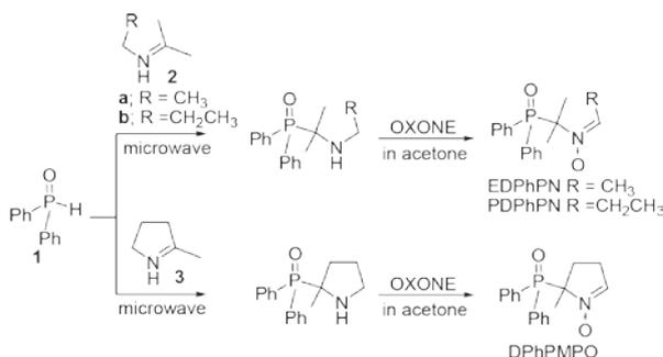
Scheme 1 Synthesis of DPhPMPO using microwave irradiation.
