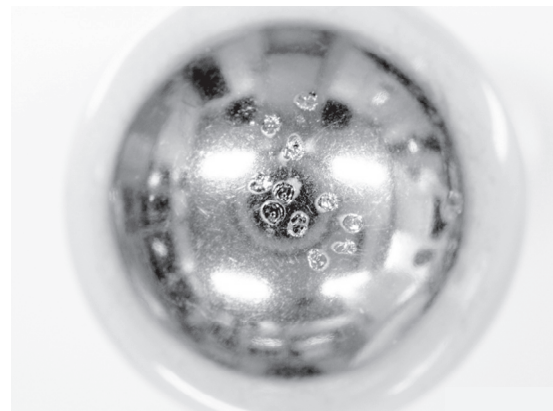
(b) High voltage electrode of 2.50 mm gap length
