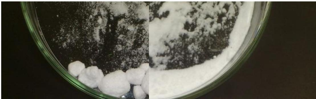
Fig.2-7 Appearance of spray dried particles
