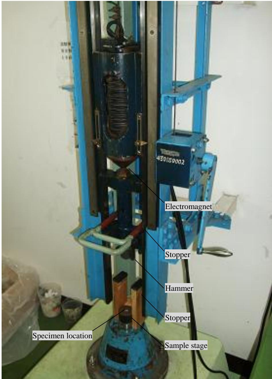
Fig.5-3 Experimental apparatus of the drop hammer sensitivity test
