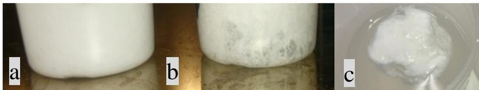
Fig.3-12 Appearance of AN-Latex mixed dispersion heated at 90 °C by constant temperature oven
