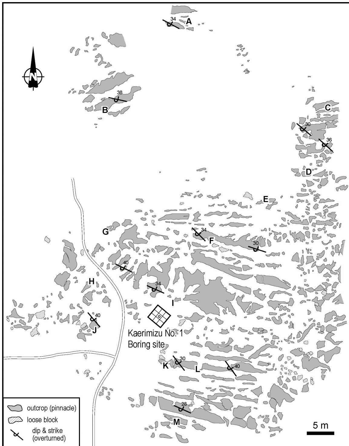
Fig. 3. Distributions of limestone outcrops (pinnacles or “lapies”) in study area, with indications of dips and strikes of strata. A to M indicate locations of outcrops described and illustrated in text.
