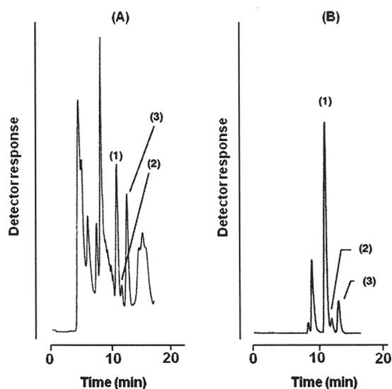
*Figure 1.* Chromatograms detected at 391 nm (A) and at 600 nm (B), which were obtained with urine spiked with PQ, DQ and IS (5  $\mu$ g/ml). Peaks: 1, PQ; 2, DQ; 3, IS; others, endogenous compounds.
