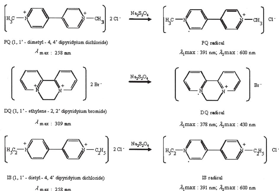
Figure 2. General scheme of the radicals from PQ, DQ, and IS by reduction with alkaline sodium hydrosulfite solution.
