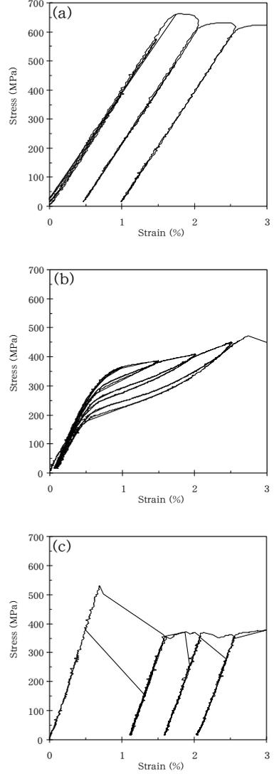
Fig. 6. Stress-strain curves given by the repeated tensile test along (a) the  $\langle 100 \rangle$ , (b)  $\langle 110 \rangle$ , and (c)  $\langle 111 \rangle$  directions.
