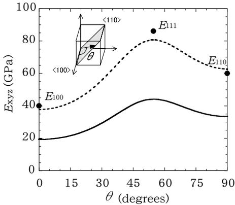
Fig. 7. Young's modulus with respect to the  $[xyz]$  direction on the  $(0\bar{1}1)$  plane.
