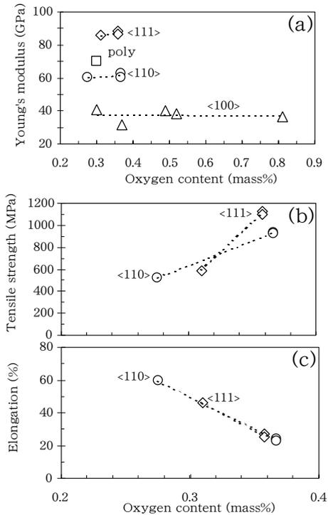
Fig. 8. All obtained (a) Young's moduli, (b) strengths, (c) elongations with respect to the concentration.
