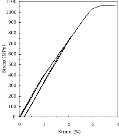
Fig. 5. A stress-strain curve obtained from the repeated compression test along the  $\langle 100 \rangle$  direction.
