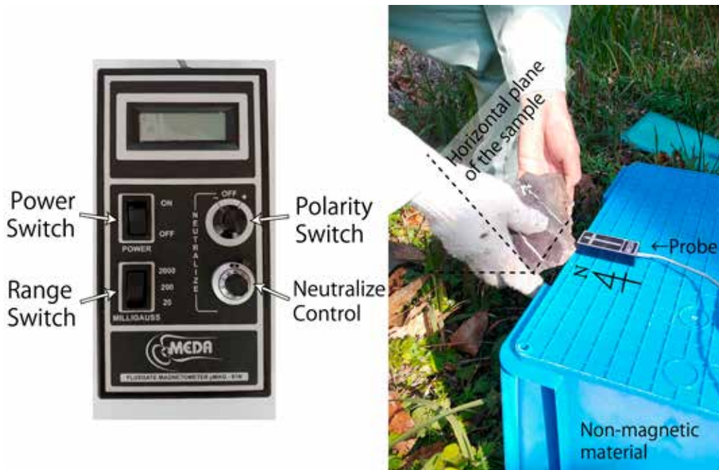
Fig. 3 Photographs showing a device (left) and its setting (right) for measuring paleomagnetic direction in the field.
