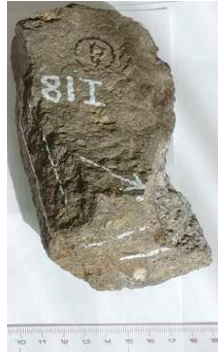
Fig. 2 Photograph of an oriented hand specimen for measurement of paleomagnetic direction. Horizontal lines on two planes and an arrow indicating the magnetic north were drawn before sampling.
